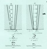
• Since the variable bandwidth tuning (VBT) filter and IF shift are separately adjustable in the TS-830S a highly sophisticated unwanted signal rejection technique may be employed: first an appropriate bandwidth is selected by the variable bandwidth tuning and then an optimum tuning point is determined by means of an IF shift.
